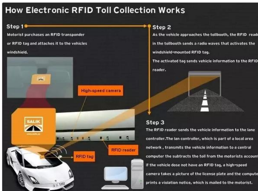
Fig 4: Working of RFID Toll Collection
